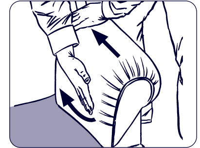
5 Using both hands simultaneously, smooth the arm cap fabric backwards and diagonally down towards the corner of the back cushion and seat platform.
